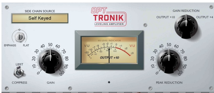
OptTronik – Based on a legendary tube-driven, electro-optical compressor, OptTronik offers smooth, musical compression with easy to use controls. The Limit/Compress switch is used to set the compression ratio and amount of compression is determined by the Peak Reduction control. The Gain control can be used to restore any volume lost to compression. The Emphasis control is used to set the high frequency response of the compressor.
