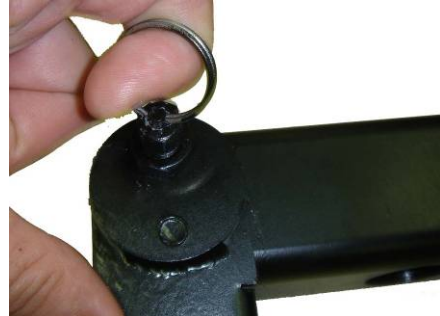
(2) Release pivoting arm locking pin
