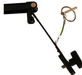
(2) Remove locking pin on the pivoting arm
