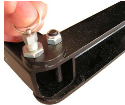
(4) Release pivoting arm locking pin
